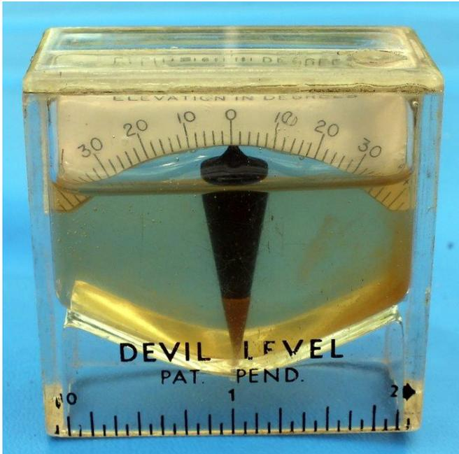
At the bottom the container is triangle shaped to put it on a pipe.
