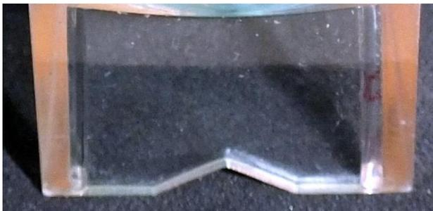
It is filled with a liquid, perhaps a kind of oil or anti freezing liquid. (In the patent description **Glycerin** is mentioned)
