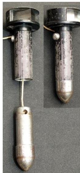
(Fig. left) And a 90 degree mirror with inserted plumb bob for surveyors.
