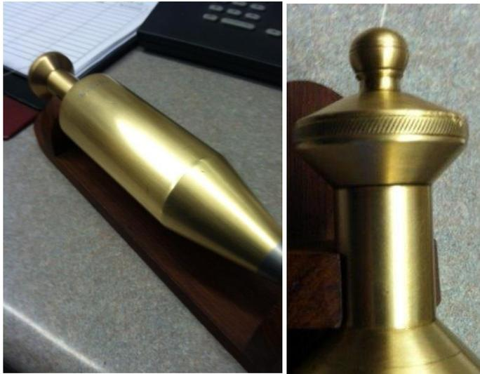
FOR THIS REASON THE MERCURY SHOULD BE SECURED BY A SECOND SCREW (LIKE IN YOUR CASE). SO THE MERCURY CAN NOT SPILL, WHEN YOU UNSCREW THE HEAD TO CHANGE THE CORD.
