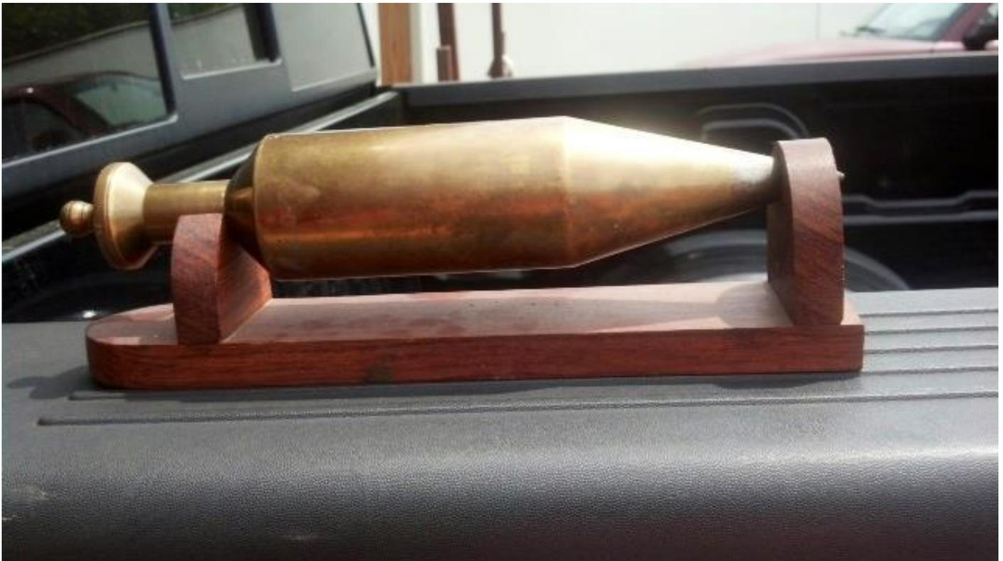
wanted it to weigh **five pounds** and he would like it to be **mercury filled** so it would settle and not be blown by the wind. This is what he built for him and it is indeed mercury filled.
