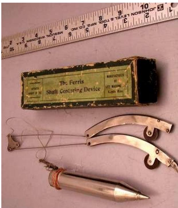
Patent US953131 FERRIS 1910 shaft centering for plumb bobs
