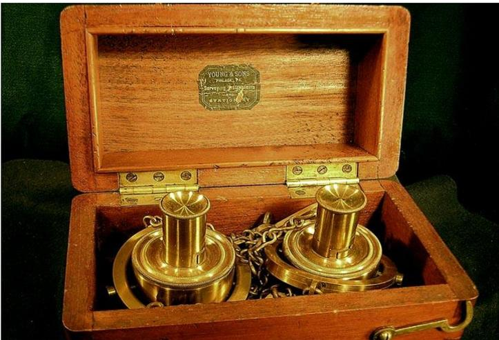
The level and compass of German mining surveyors are stored in wooden boxes to avoid electric sparks in the mines. From my collection.
