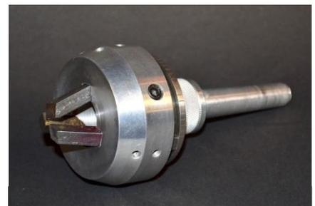
Tailstock mounted adjustable hollow mill. The 3 cutters are advanced simultaneously by a threaded ring so that once adjusted it allows me to repeatedly reduce the diameter of rod stock to a specific diameter without having to stop the lathe and check the progress with the digital caliper
