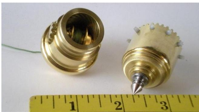
internal reel on spring loaded pinion gear shaft
