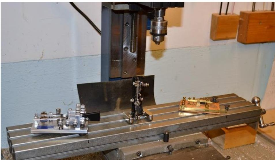
3 miniature telegraph keys on the milling machine table.
