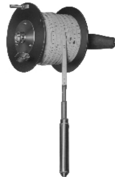
Water Level Meter ("Kabellichtlot") made in 1962
