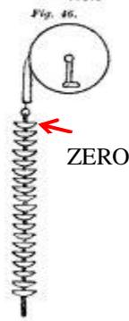
**1895** <sup>14</sup>: The measurement of the ground-water, best indicated by the height of the water-level in wells. Pettenkofer uses **a rod for shallow wells and a cord for deep wells** to which are **attached a number of little cups** which are let down into the well and drawn up again.
