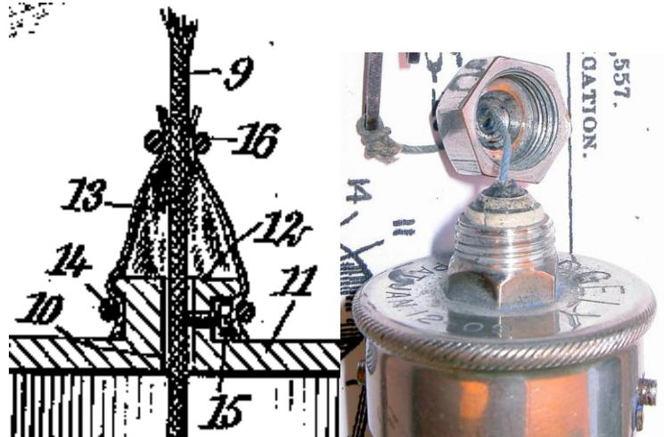
**Inside** the line is fixed to the axle by a screw.
