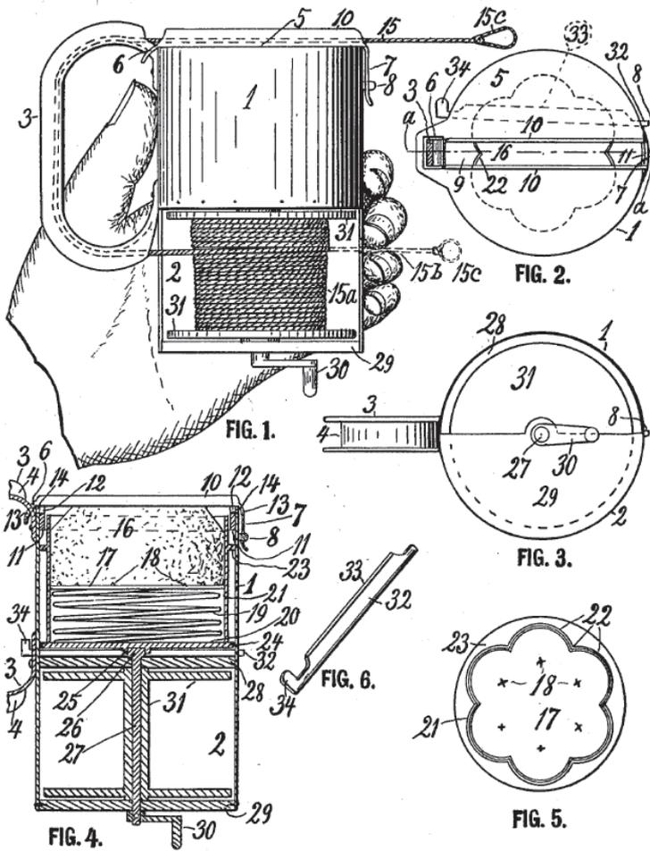
My invention relates to chalk-line holders, and the object is to provide an efficient device for holding and chalking the string or cord used by carpenters and others for marking straight lines.
