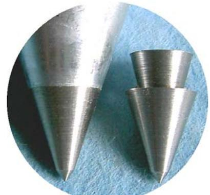
Since the plumb bob needs to be fashioned into a symmetrical shape and a string has to be attached to the bob’s axis of symmetry, the workability of the base material is significant as is the technology available to shape the material. Thus, as tooling became available to cast iron and machine steel, these materials became an alternative to brass or were used to fashion certain parts of the plumb bob, such as the delicate tip.
