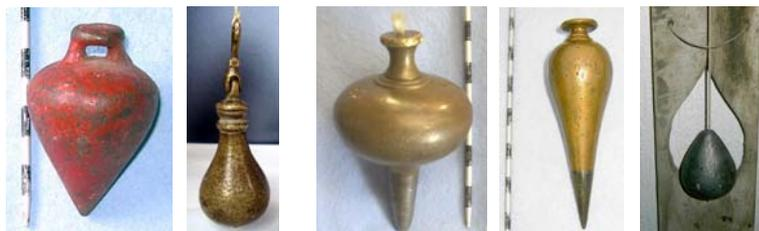
“**Geometric**”: Shapes often used and modified are the cylinder, cone, sphere or a combination of shapes such as the pencil point, tapered cylinder, hexagonal cylinder, ice cream cone, bullet.
