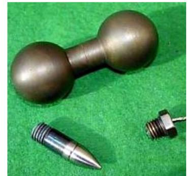
Less frequently used, dense but malleable materials are hardwoods, bone, ivory, and mercury encapsulated in a jacket of steel or brass.
