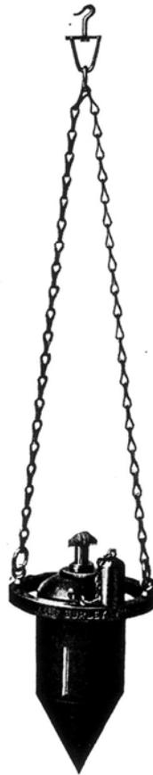
THE PLUMMET LAMP, No. 170, is a large plummet, of which the upper part is hollow to contain oil. It has a tube with a wick, and an extinguisher.
