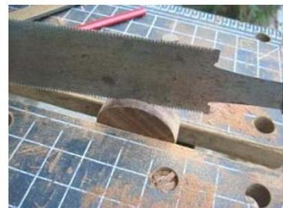
Cutting the groove in the wheel
