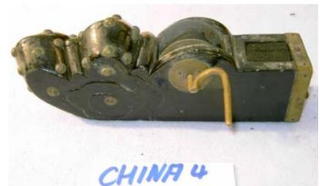
C3 c) Later chalk boxes were produced from brass. The shape was a pot with a reel attached to the side.
