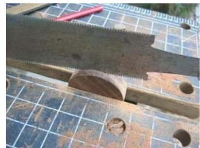
Cutting the groove in the wheel
