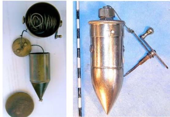
C5 b) To draw longer lines more useful to the mason or carpenter, larger reservoirs for the chalk were fashioned which when shaped symmetrically with a tip, serve a legitimate dual function of combining chalk box with plumb bob.
