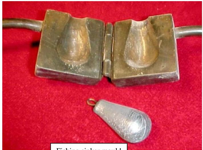
Fishing sinker mould
