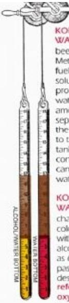
**KOLOR KUT MODIFIED WATER FINDING PASTE** has been designed for use in Methanol, Ethanol enriched fuel systems. Alcohols are soluble in fuels in all proportions when they are water-free but relatively small amounts of water can cause separation of alcohol from the fuel. The mixture settling to the bottom of the storage tank contains a high concentration of alcohol and cannot be detected by most water detection pastes.
