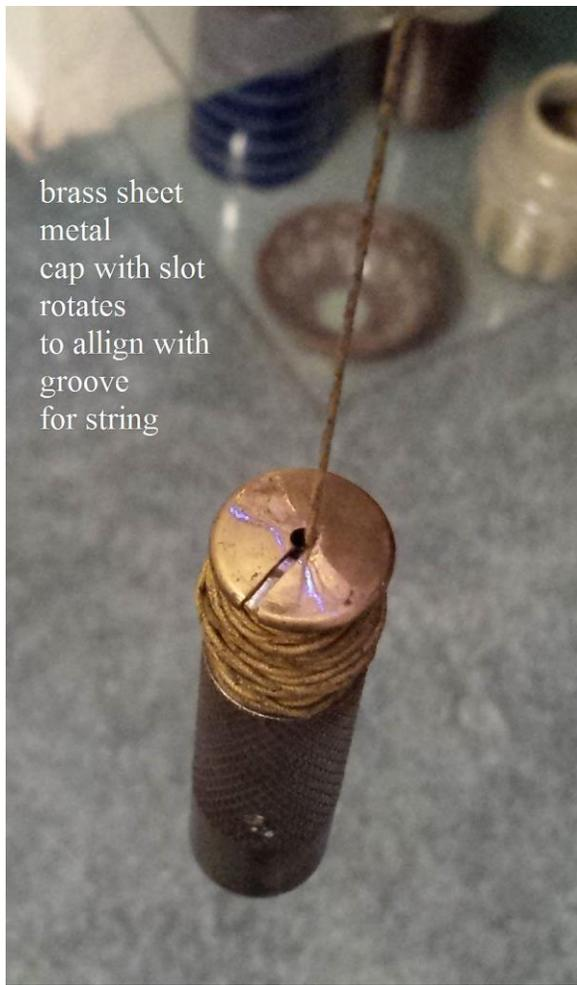
brass sheet metal cap with slot rotates to align with groove for string
